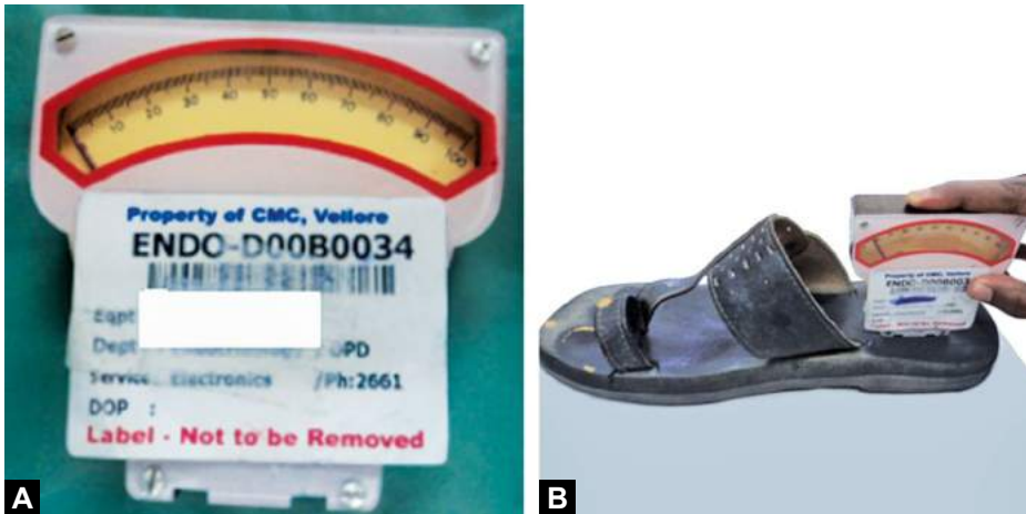
Figs. 12.10A and B: (A) Durometer; (B) Checking the shore value of the footwear.
