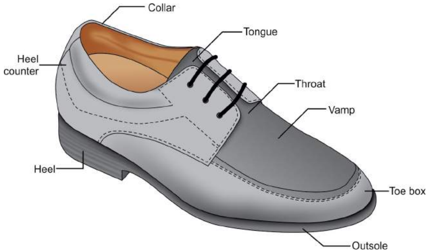
Fig. 12.8: Parts of footwear.
