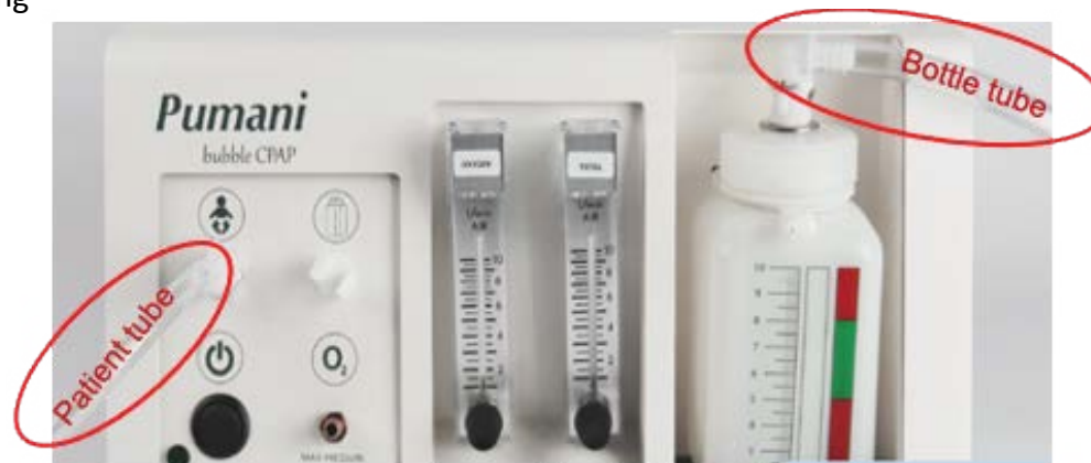
Fig 2.3.5c Connect the Patient & Bottle tubings to the machine
