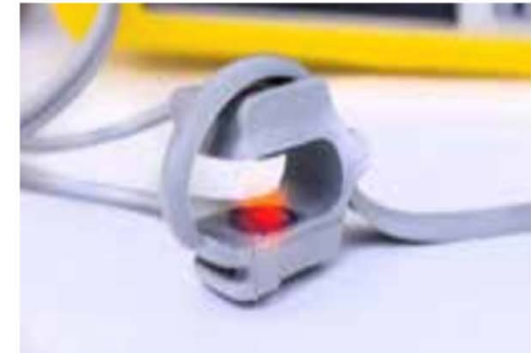
Fig 2.6.5c Check for red light on sensor
