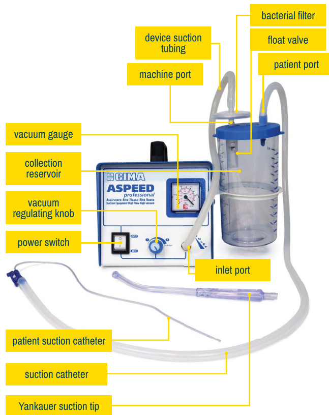
Fig 2.2.5 Parts of the Suction Machine
