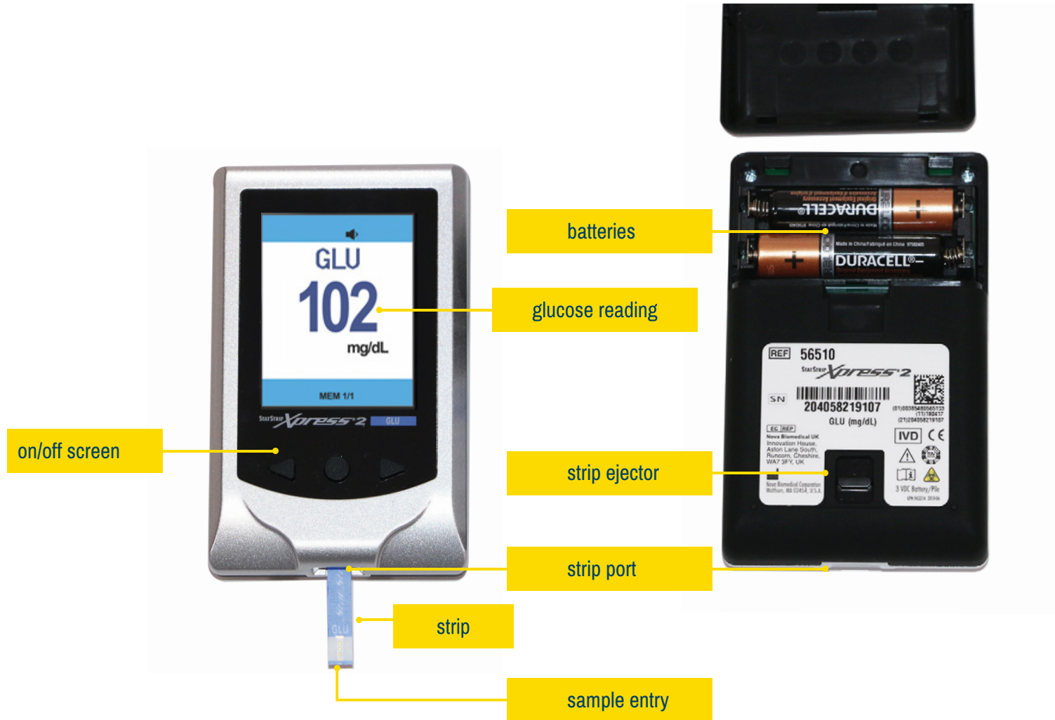
Fig 2.8.4 Parts of a glucometer
