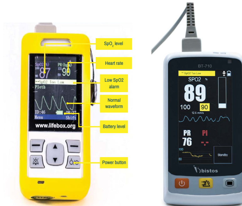
Fig 2.6.4 Parts of a Pulse Oximeter
