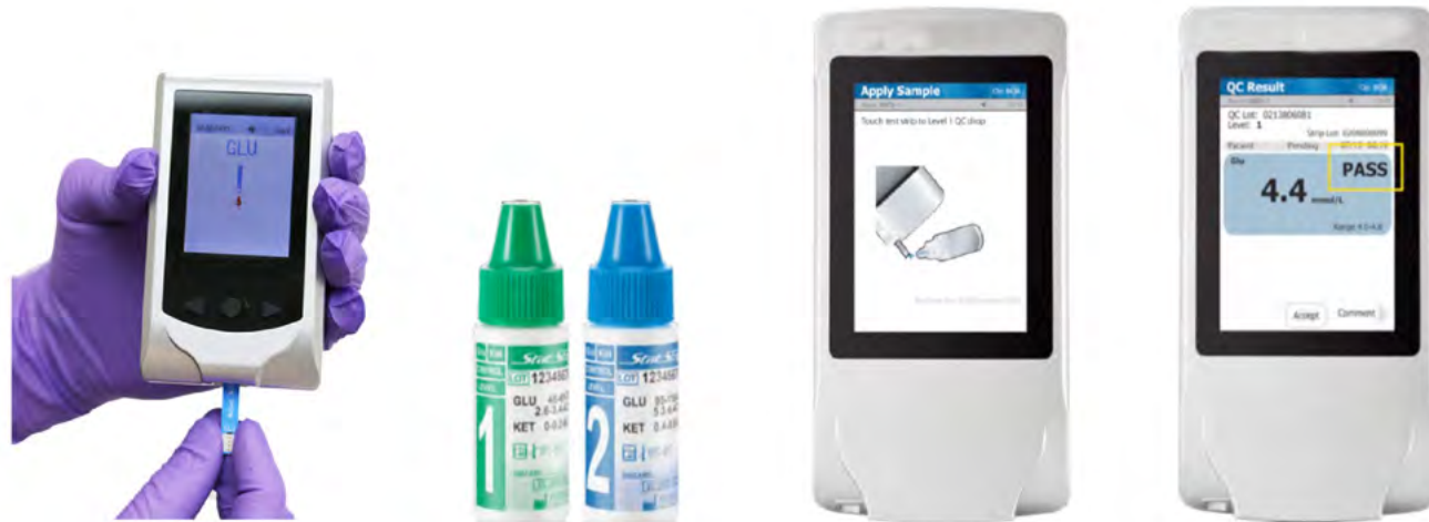
Fig 2.8.5b Insert strip, place control solution on strip, wait a few seconds, PASS result will show
