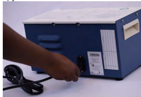
Fig 2.3.5a Place the Pumani CPAP on a firm surface allowing airflow through the vents and connect to power
