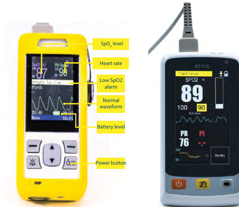
Fig 2.6.4 Parts of a Pulse Oximeter
