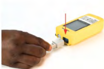
Fig 2.6.5a Connect the probe
