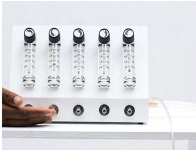
Fig 2.5.5 Confirm oxygen is flowing by feeling for air flow on each of the splitter outlets
