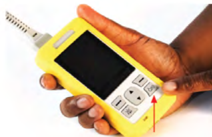
Fig 2.6.5b Turn the Oximeter On
