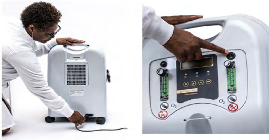
Fig 2.4.5a Plug concentrator into a power source and turn on
