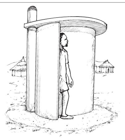
VIP latrines may be designed with single or double pits. Double pits may be used, for example, when cultural taboos prohibit the mixing of male and female faeces. Twin pits may also be used to facilitate emptying and composting. When one pit is full, the other can be emptied and reused. The pit of a VIP latrine is usually located directly beneath the slab to prevent fouling of the chute, which would lead to odour and fly problems, and require regular cleaning.
