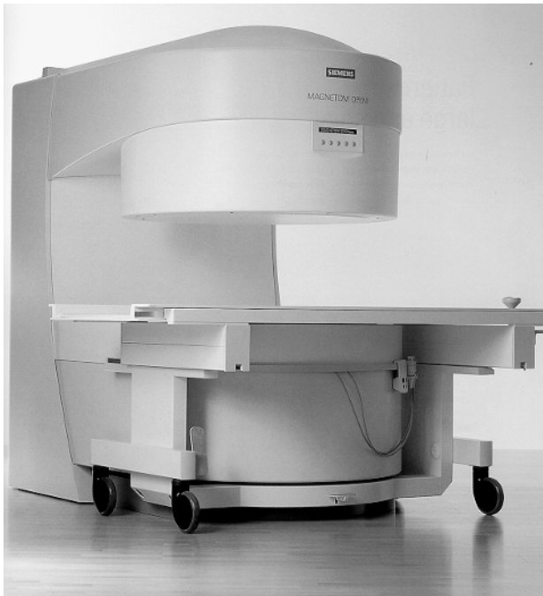
Figure 6.23 An example of an open magnet system. The main field is produced by a large diameter electromagnet/iron pole with the pole gap arranged vertically across the patient table. The field in this case is 0.2 T. (Siemens).
