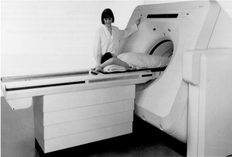
Figure 4.21 A Modern CT Scanner: The X-ray tube and detectors rotate within the square enclosure. During the course of the scan the motorised and position-encoded patient bed is moved through the large hole. This lateral movement achieves slice selection. Generally the scanner housing can be tilted \pm 30^\circ with respect to the horizontal to allow slices at different angles to the patient to be obtained. (Courtesy of Siemens UK Ltd).
