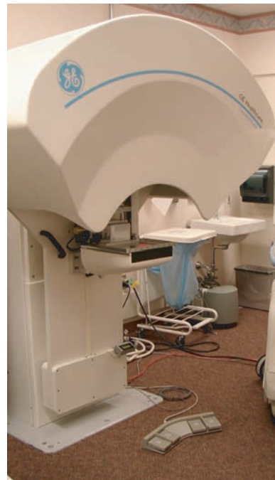
Figure 3.25 Second generation Digital Breast Tomosynthesis prototype installed at the University of Michigan for clinical research. (Courtesy of GE Healthcare.)
