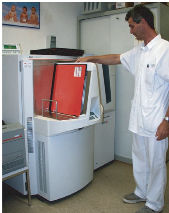
Figure 2.6 This system scans the latent image with a laser beam and erases the residual image on the storage phosphor after which the screen can be reused for new X-ray exposure.
