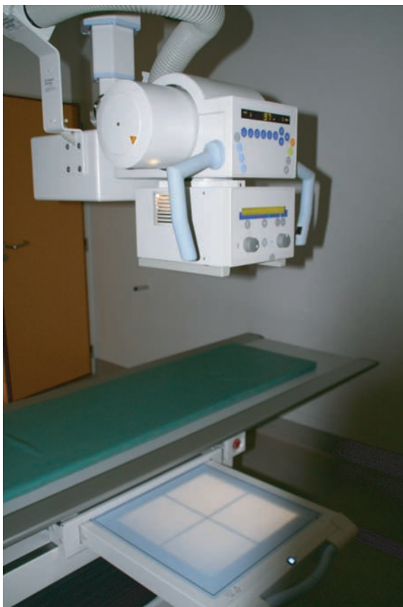
Figure 2.11 In more recent X-ray systems the cassette and image intensifier are replaced by an active matrix flat panel detector. This picture shows a Siemens system with large-area amorphous silicon detector coupled to a CsI scintillator plate.
