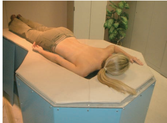
Figure 3.32 Breast CT prototype by John Boone et al. The patient is placed in prone position and the X-ray tube and detector rotate around the pendant breast. (Courtesy of UC Davis Health Systems.)
