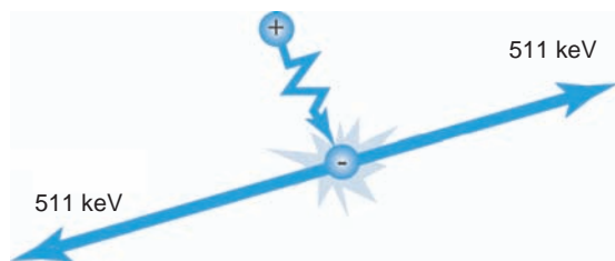
Figure 5.1 Schematic representation of a positron–electron annihilation. When a positron comes in the neighborhood of an electron, the two particles are converted into a pair of photons, each of 511 keV, which travel in opposite directions.
